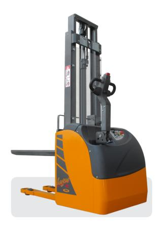
Versatile and manoeuvrable, Logos ac is the ideal pedestrian operated lift truck for standard applications. It has been completely renewed with a 0.7 kW ac traction motor and a high level electronic control which grant manoeuvrability and power during all working conditions to be used also on gradual ramps. The new steering system allows to make more agile manoeuvres in narrow spaces and working aisles less than 2.250 mm.
