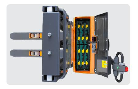
The battery compartment is easily accessed by simply lifting the hinged lid, thus facilitating daily and periodical battery checks and recharging. Focus ac is equipped with traction batteries up to 375 Ah. The wo-wa built-in charger (option) provides easy and reliable charging at any plug socket.
