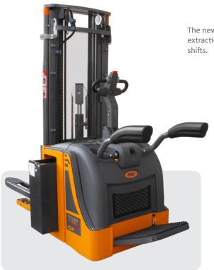
The new 716 P ac is equipped with traction battery 24V 375Ah. The side battery extraction facility, standard, is available for the operation on different working shifts.
