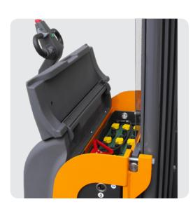
The new range of industrial stackers is equipped with traction batteries up to 375 Ah. The side battery extraction facility is available for the operation on different working shifts. The wo-wa built-in charger (option) provides easy and reliable charging at any plug socket. The electronic control is IP65 protected. As option, the electronic system on tiller arm is weatherproof IP 55 (standard for cold store execution).
